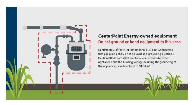
These safety hazards associated with improper bonding or grounding can result in lifethreatening circumstances.
