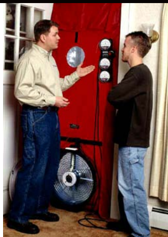
Customers appreciate the energy-saving advice they receive during a Home Energy Audit. Shown above is a blower door test, one of several high-tech components of the more in-depth audit.
