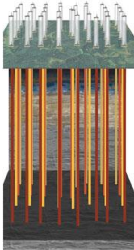
Traditional Vertical Well Spacing: 32 Separate Padsites Needed For 32 Wells. (Method not used by Chesapeake)
